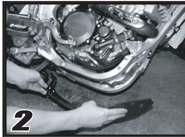
**2.** take the skidplate and pre-flex it to match the contour of the bikes engine cradle. you may find that you have to bend it beyond the arc of the frame to get it to settle to match the bikes frame.
