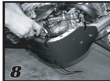
**7. & 8.** only tighten the straps after you have all 6 in place. once again tighten the straps a little bit at a time so the skidplate remains in the desired location. once the straps are tight you can trim the excess away with a pair of side cut pliers. review the installation to make sure vent lines and controls are free and clear of obstruction. you are ready to ride.
