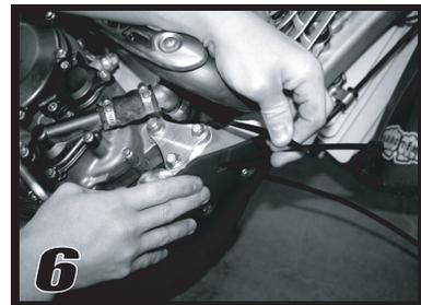
**6.** when securing with the tie straps make sure you are only around the frame not on vent lines or control cables. also positioning around engine mounts can be tricky so look over the position before securing the strap.
