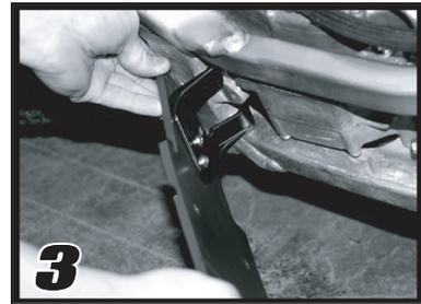
**3.** locate the frames cross member towards the back portion of the cradle. This locates the skidplate and keys it into position. put the tongue around the crossmember and pivot the skidplate upward into position.
