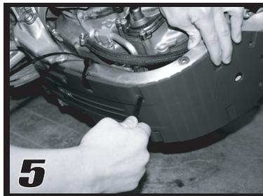
**4. & 5.** secure in place with provided tie straps. make sure you don't pull them too tight in the beginning. you will want to work from side to side and back to front. tighten the straps a little bit at a time this will allow you to position the skidplate in the desired location on the bike.
